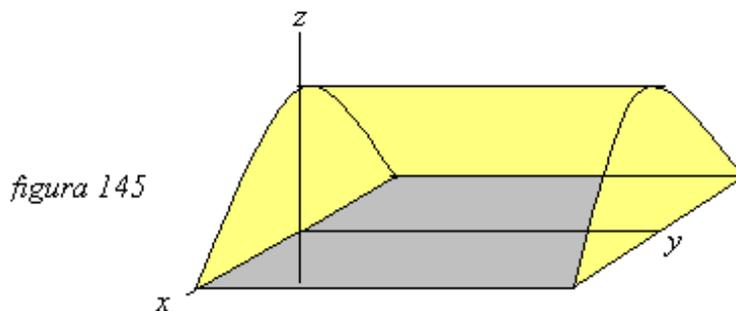
$$m(S) = \iiint_S \rho(x, y, z) dz dy dx = \int_{-2}^2 \int_0^9 \int_0^{4-x^2} x^2 dz dy dx = \frac{384}{5}$$
