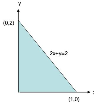
$$\iiint_S y dz dx dy = \int_0^1 \int_0^{2-2x} \int_0^{x^2+y^2+1} y dz dy dx = \int_0^2 \int_0^{\frac{2-y}{2}} \int_0^{x^2+y^2+1} y dz dx dy = \frac{23}{15}$$
