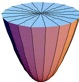
$$V = \iiint_S dz dy dx = \int_{-1}^1 \int_{-\sqrt{1-x^2}}^{\sqrt{1-x^2}} \int_{x^2+y^2}^1 dz dy dx = \int_0^{2\pi} \int_0^1 \int_{r^2}^1 r dz dr d\theta = \frac{1}{2}\pi.$$
