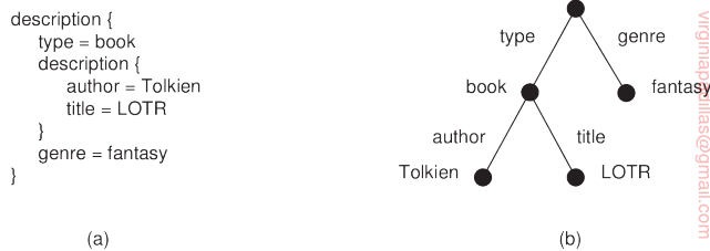
Figure 5.31: (a) A general description of a resource. (b) Its representation as an AVTree.
